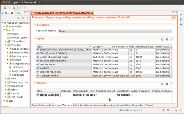
**Figure 5.** Input flows in the biogas upgrading infrastructure process generated in openLCA. There is a single output - one piece of upgrading plant.
