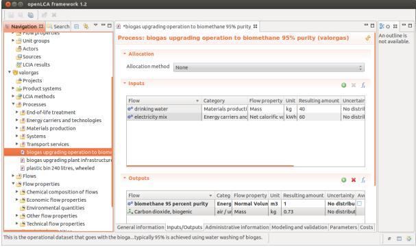
**Figure 6.** Metener gas upgrading operational process dataset in openLCA 1.2.9 using the ELCD version 3 database. Two inputs and two outputs are modelled
