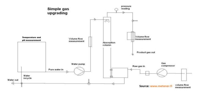
**Figure 4.** Flow diagram of Metener type water scrubbing rig in 2011 involving a water column. Source: http://www.metener.fi.
